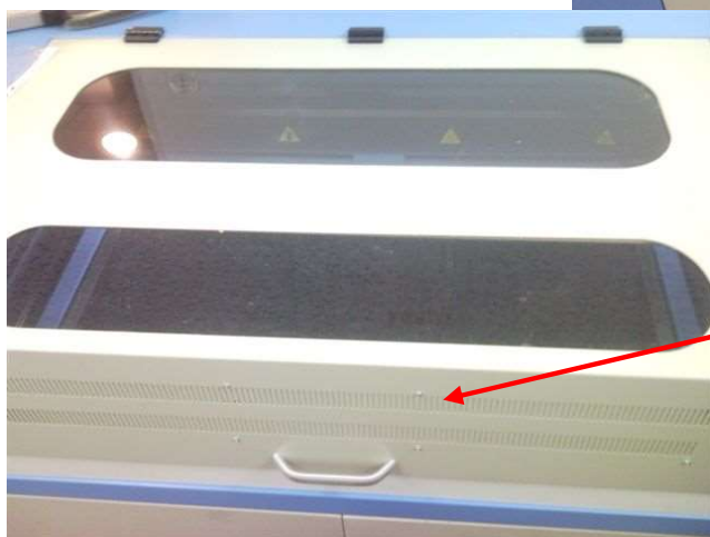
Door With blocking of stray light & spacers for Ventilation
